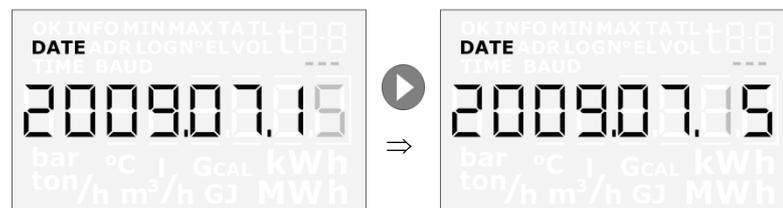
The active digit flashes and this digit can be changed by pressing the subkey. You go from the leftmost to the rightmost digit by pressing the main key.
