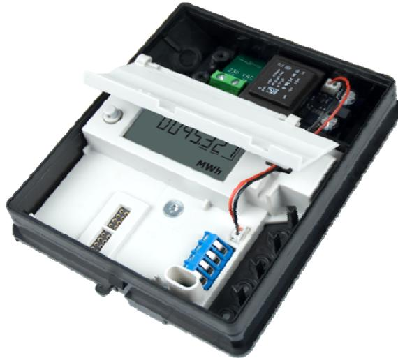
National regulations for electric installations must be observed. The 230 VAC module can be connected/disconnected by the utility’s personnel, whereas the fixed 230 V installation into the meter panel must be carried out by an authorized electrician.
