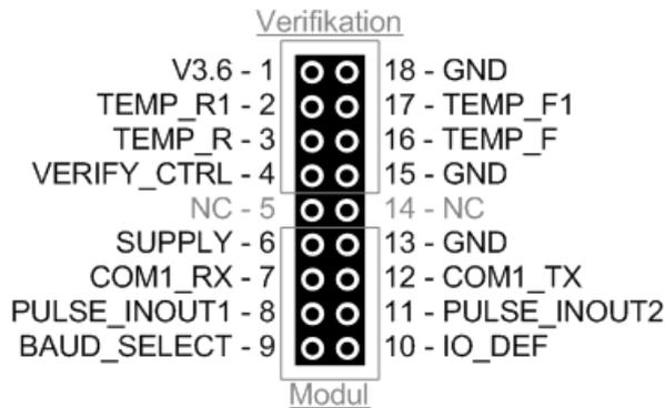
The upper part of the connector is used for ”verification”. This part is normally sealed to prevent inadvertent access.
