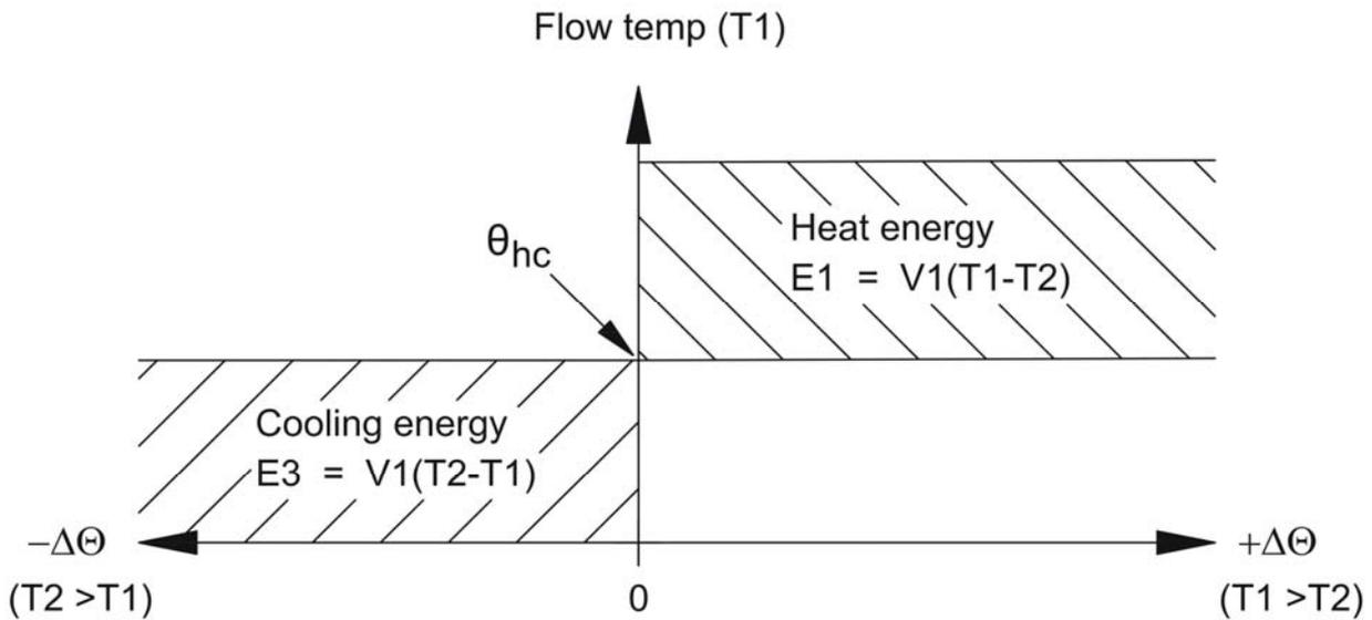
If the current T1 exceeds, or equals  $\theta_{hc}$  only heat energy can be measured. If the current T1 is lower than or equals  $\theta_{hc}$  only cooling energy can be measured.
