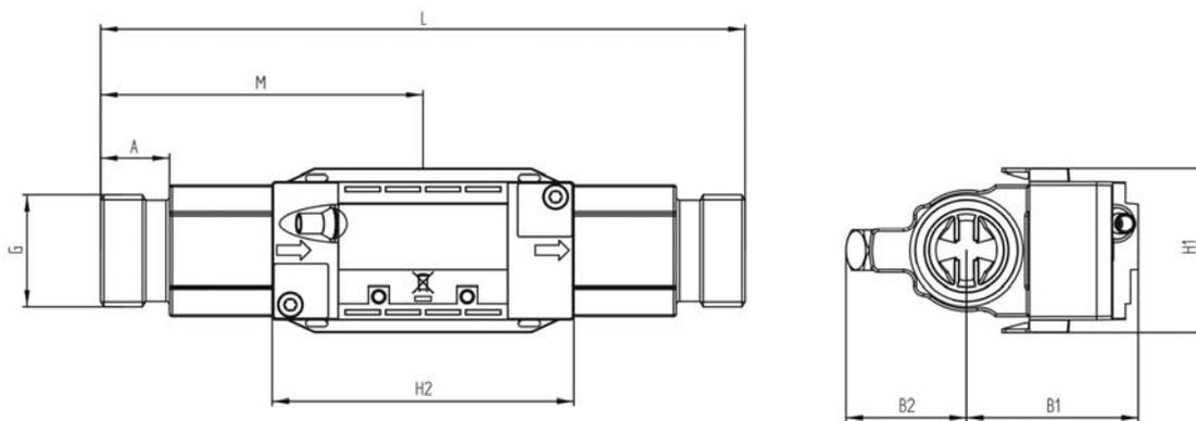
Figure 3: Flow sensor with G<sup>3</sup>/<sub>4</sub> and G1 thread connection
