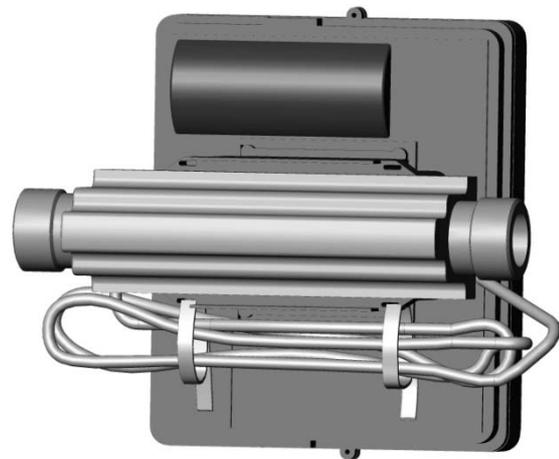
Figure 15: Fastening of cable
