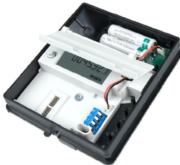
Note: AA-cell lithium batteries include approx. 0.7 g lithium each and are therefore not comprised by transport restrictions.
