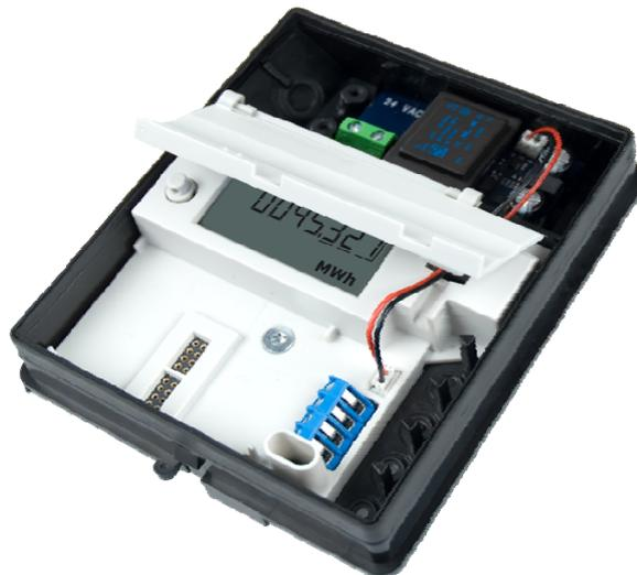
National regulations for electric installations must be observed. The 24 VAC module can be connected/disconnected by the heating station’s personnel, whereas the fixed 230/24 V installation in the meter panel must only be carried out by an authorized electrician.
