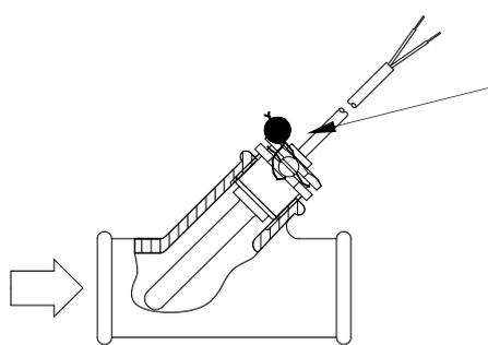
The plastic tube on the sensor cable is placed on a level with the sealing screw, which is lightly tightened with your fingers.
