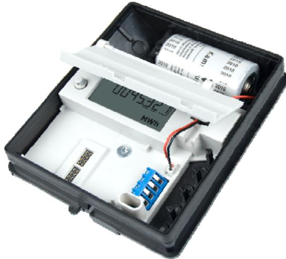
Note: D-cell lithium batteries include approx. 4.5 g lithium each and are therefore comprised by transport restrictions. See document 5510-408\_DK-GB-DE for further details on transportation of lithium batteries.
