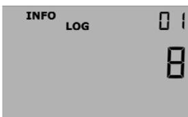
...next the information code set on this date is displayed. In this case there has been a sensor error in temperature sensor T1 on 4 January 2010.
