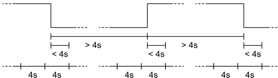
At the very moment PULSE-INOUT1 is connected the verification registers are reset. Maximum 4 seconds after this the verification registers are counted the first time followed by normal counting in the registers every 4 seconds.
