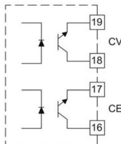
The pulse outputs are designed with darlington optocouplers, which makes them suitable for most signal types. Please note the polarity when making the connection. See paragraph 2.2 re electrical data of the pulse outputs.
