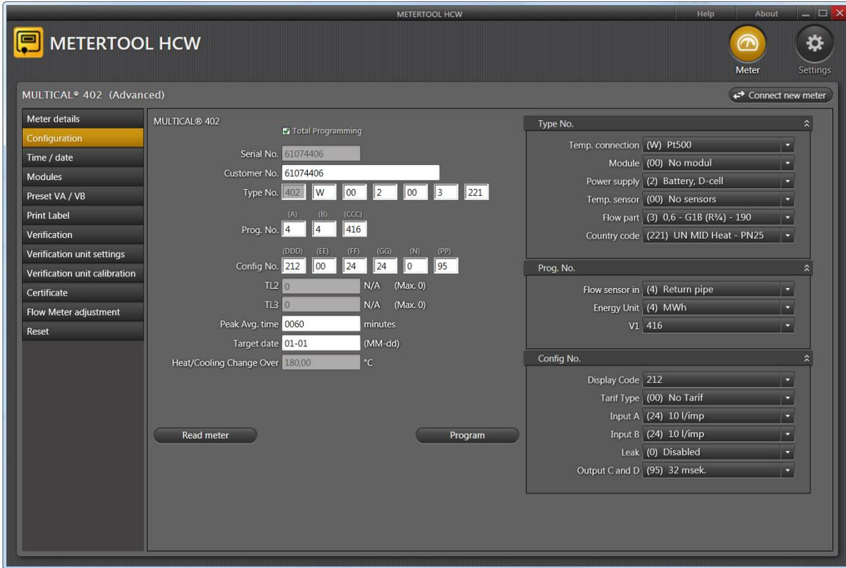
The configuration of MULTICAL® 402 can be read out directly. The program is self-explanatory as to most coding numbers (see text in "combo-boxes"), further details can be found in the respective paragraphs of the technical description.
